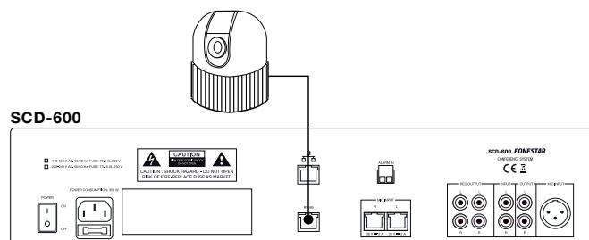
There are 2 types of connection: direct support of the PELCO-D protocol directly (RS-485); and VISCA protocol (requires an RS-485 to RS-232 converter).
