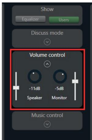
Allows you to change the volume of the system's audio outputs:
