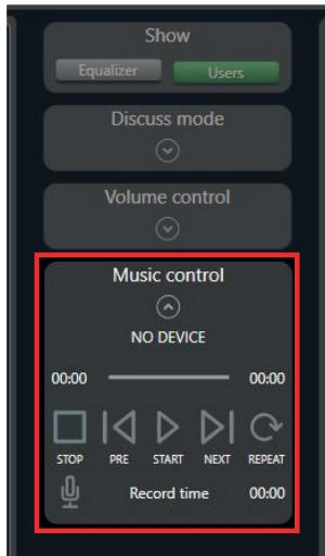
The software allows you to control playback or recording of the USB device connected to the front panel.
