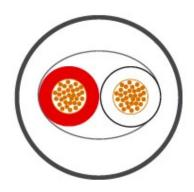
OFC cable with double insulation
