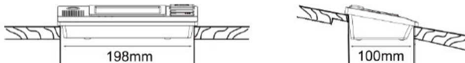
Figure 4 Schematic Diagram of Creating a Slot for Seating the ZS-200M (Level Surface)
