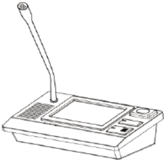
Figure 7 Microphone Pole Installation Diagram
