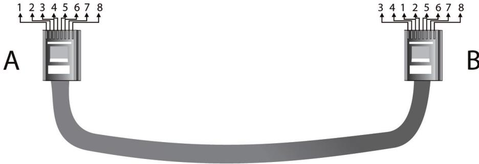
The connection between the microphone and the PA system or several microphones in cascade must be made using a Cat 5e or Cat 6 cable. This cable consists of 8 conductors which must be connected according to the diagram above and finished at both ends with RJ-45 (8P8C) connectors.
